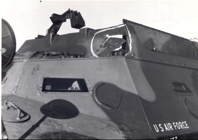
XM-706 damaged by B-40 rocket during attack on Phan Rang AB (Air Force Historical Research Agency)
